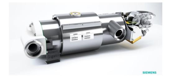
**Figure 54** Siemens angiography tube of the Gigalix<sup>TM</sup>series, launched 2013, with grid switchable flat electron emitter and liquid bearing. (Picture courtesy of Siemens.)
