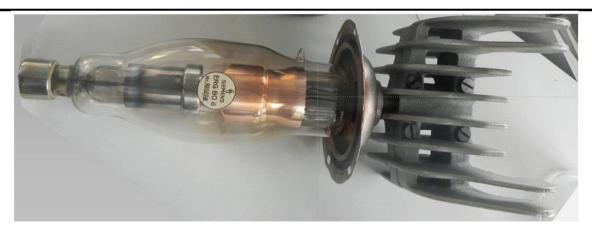
Figure 23 Siemens stationary anode tube ERG 80 ö with cooling fins from 1942. (Photo taken in the Siemens X-ray tube museum Rudolstadt, Germany.)
