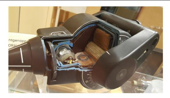
**Figure 47** Cut-off picture of a Philips Oralix<sup>TM</sup> dental tube head. Tube current and focal spot size were stabilized with a Wehnelt electrode and self-controlled resistive biasing. (Picture taken at the Medizinhistorisches Museum Hamburg, Germany,UKE.)
