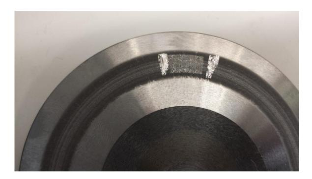
**Figure 22** Eroded focal track of a rotating anode. Malfunction of the rotor during two subsequent trials to rotate caused two marks of molten target material (the marks map the shape of the rectangular electronic focal spot).
