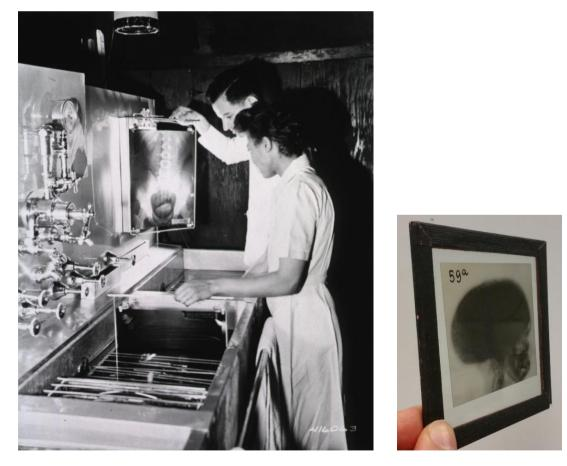
Figure 4.a Radiographs recorded on a glass plates being chemically processed. They are rigid, fragile, and relatively heavy to handle b. An early radiograph recorded on a glass plate.
