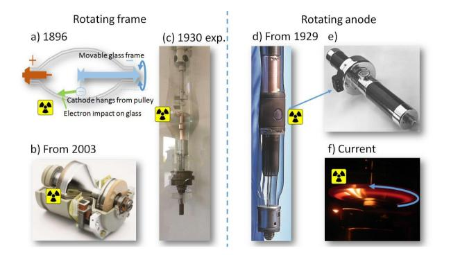
Figure 12 Competing concepts. Left: rotating frame, right rotating anode tubes:
