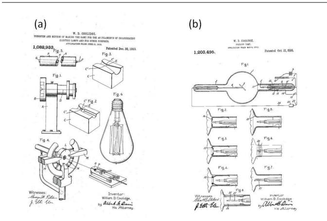
**Figure 9** Photo of the illustration page of W.D. Coolidge's patent for the production of ductile tungsten, US1082933, filed in 1912. (Source: https://patentimages.storage.googleapis.com/pages/US1082933-0.png, accessed October 12<sup>th</sup>, 2017). (b) Photo of the 1913 patent of Coolidge for the hot cathode high vacuum x-ray tube.
