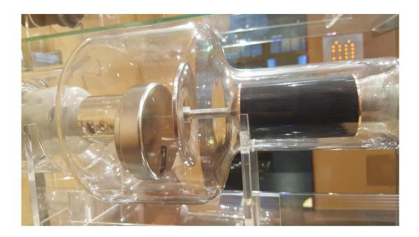
**Figure 31** Hidden cathode in a Philips tube from the production plant in Eindhoven, The Netherlands. (Picture taken at the Medizinhistorisches Museum Hamburg, Germany,UKE.)
