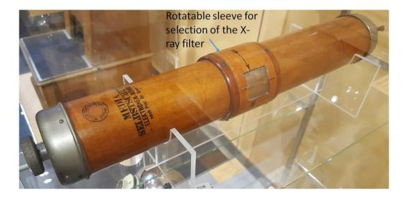
**Figure 14** "Fully protected" Philips Media<sup>TM</sup> tube from the 1920ies. A rotatable sleeve allowed for selecting the X-ray filter thickness. (Photo taken at the Medizinhistorisches Museum Hamburg, Germany, UKE.)
