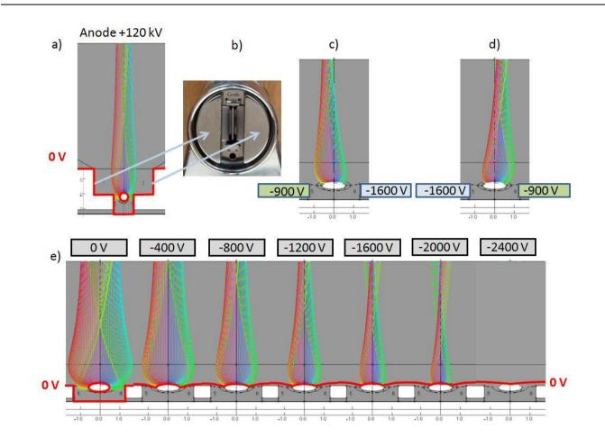
**Figure 52** Ray tracing of electrons. Planar cross section through the emitter coil. Biasing of the control electrodes allow for focal spot deflection, as used in CT application, and also for switching the electron beam off.
