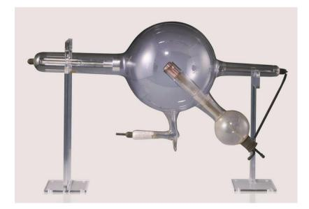
**Figure 7** Toshiba "Giba" x-ray tube, the first Japanese domestic x-ray tube, developed and commercialized in 1915by Toshiba Denki, later Toshiba Electron tubes & Device Co., Ltd (TETD, now Canon, Japan, group). Many types of x-ray tubes have been developed originating from this "Giba X-ray tube". (Courtesy of Toshiba Science Museum.)
