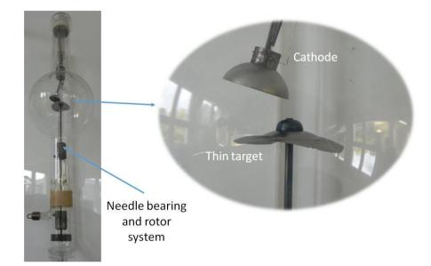
**Figure 16** Experimental rotating target tube from 1927 by PhönixRöntgenröhrenfabriken AG, Rudolstadt, Germany, later Siemens. (Picture taken in the Siemens X-ray tube museum Rudolstadt, Germany.)
