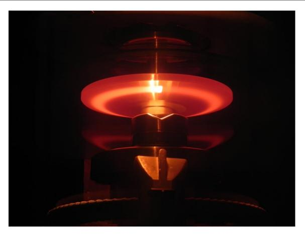
**Figure 19** Thermal picture of a rotating anode tube during the exhaust process. The rectangular thermal focal spot and the hot trail of the focal track are visible on top of the light from the filament of the cathode at the bottom, reflected from the anode.
