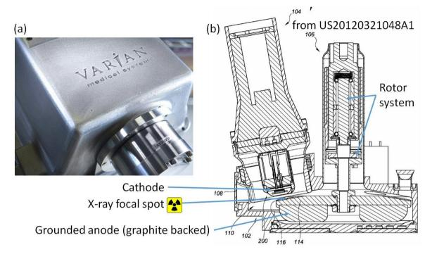
**Figure 55** (a) Logo on one of the first anode end grounded (AEG) tubes developed by Varian, now Varex, Salt Lake City, UT, USA. (b) Drawing of an AEG tube frompatent application US20120321048A1. (Picture (a) courtesy of Varex.)
