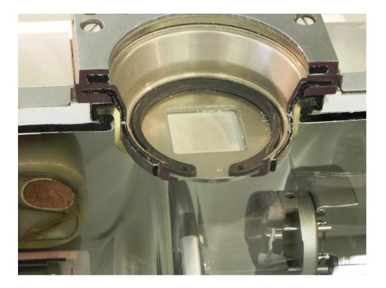
**Figure 38** Close-up view of the radiation port of a Philips tube housing assembly for radiography and angiography with exchangeable near focal spot apertureagainst off-focal radiation and intrinsic radiation filter.
