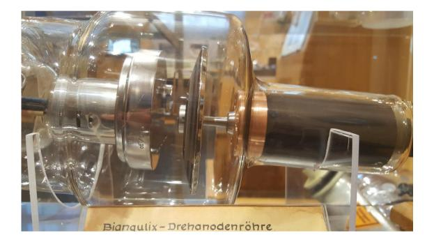
**Figure 18** Siemens Biangulix<sup>TM</sup> tube. Its anode has two separated focal spot tracks with different anode angles. (Picture taken at the Medizinhistorisches Museum Hamburg, Germany,UKE.)
