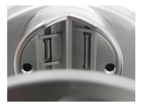
Figure 32 Close-up view of the thermionic cathode for superimposed focal spots of a Philips SRO<sup>TM</sup> 33 100 tube.
