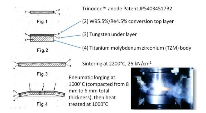
Figure 26 Philips Trinodex<sup>™</sup> anode, in production from 1973, hot forged from three metal slabs.
