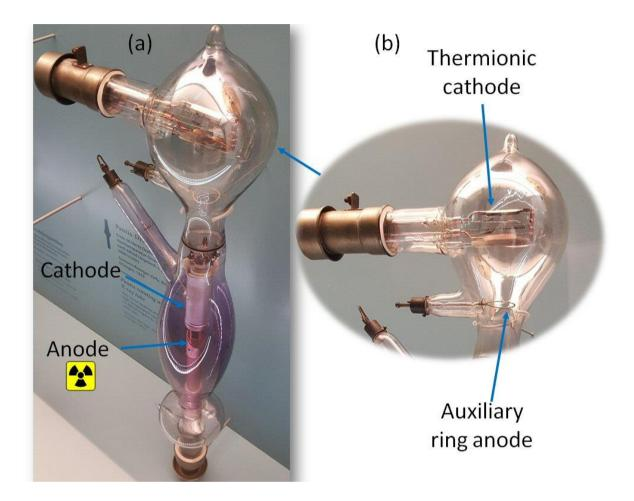
**Figure 8** (a) Lilienfeld ion X-ray tube with thermionic electron production to pre-ionize residual gas. (b) Thermionic electron X-ray "softener", an electron source with auxiliary anode to pre-ionize the residual gas. This model marks the transition between ion tubes and high vacuum tubes. (Photo taken at the German Röntgen Museum, Remscheid-Lennep, Germany.)
