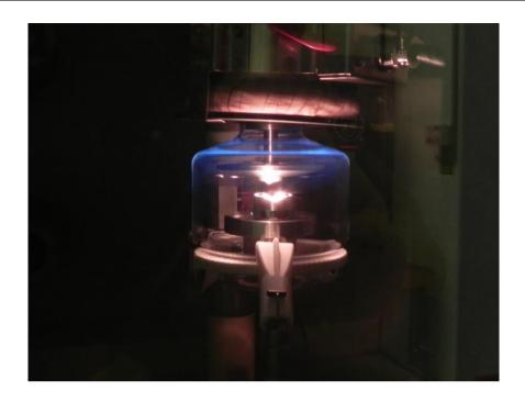
**Figure 39** Photo of a glass tube during the exhaust process with electron bombardment of the anode. The blue glow at the inner glass wall (top, about the cathode region) signalscontinued impact of backscattered electrons and ionson the glass.
