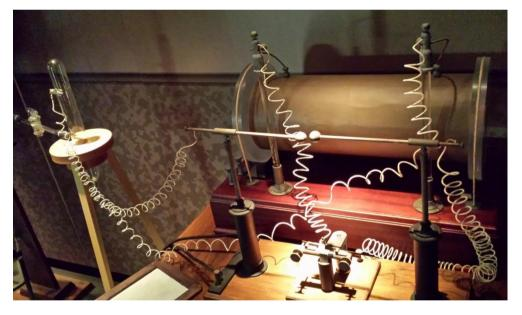
**Figure 1** Replica of C.W. Röntgen's first experimental equipment in his laboratory in Würzburg, Germany. It shows an actively pumped simple Crookes tube and a "large" Rühmkorff inductor. Röntgen discovered X-rays at dawn of Friday November 8<sup>th</sup>, 1895. (Photo taken at the German Röntgen Museum, Remscheid-Lennep, Germany.)
