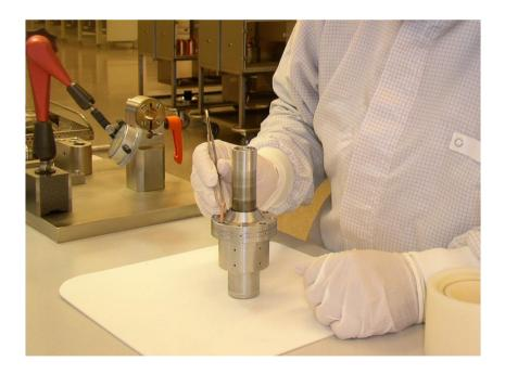
Figure 35 Final assembly of a liquid metal bearing system for the Philips MRC<sup>TM</sup> 200 angiography tube series.
