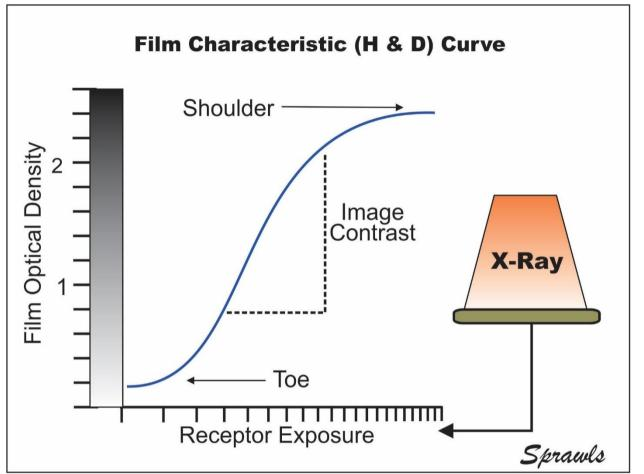
Figure 5. The characteristic (H & D) curve relating film 0ptical density to receptor exposure that is on a logarithmic scale.
