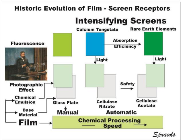
Figure 2. The major phases in the development and evolution of film-screen radiographic receptors.
