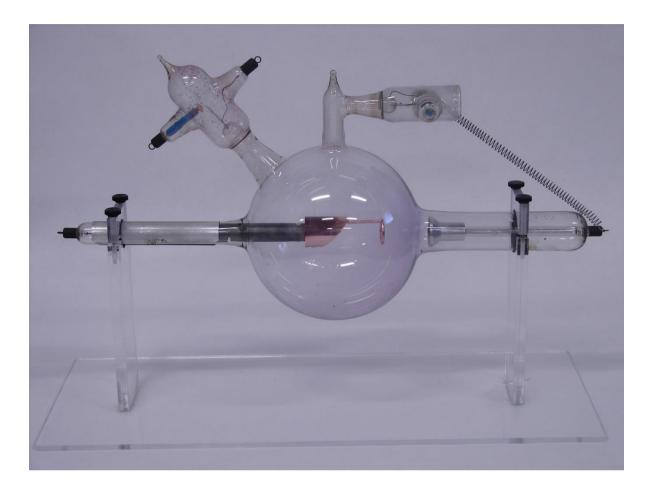
**Figure 27** Hydrogen ion X-ray tube with field enhancing pull ring on anode potential, introduced in 1916 by the Victor X-Ray Company of Chicago, IL, later to be acquired by General Electric to become GEXCO, the forerunner of today's GE Healthcare. (Photo courtesy of GE.)
