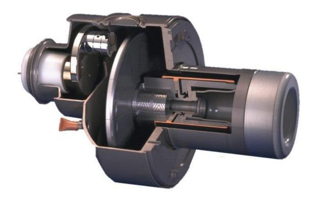
Figure 36 First rotating anode tube with liquid bearing and 200 mm anode disk, Philips  $MRC^{TM}$  200 series for cardiology and angiography.
